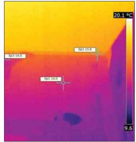
The right hand side of toggle and seat shows a greater amount of friction and therefore heat from approximately the midway position of the toggle.
