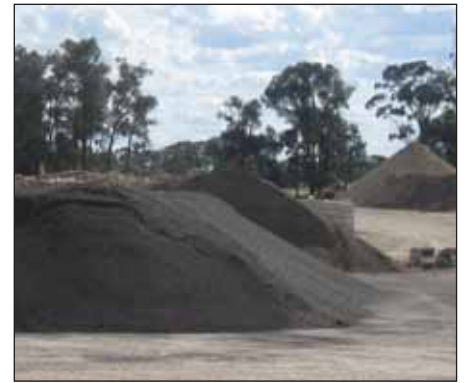
Stockpile of Recycled Asphalt Pavement
