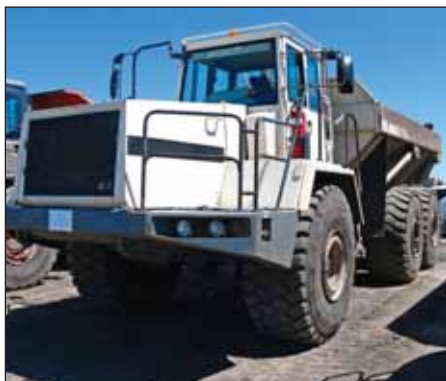
Guardrails installed beside the engine bay of an articulated dump truck provide physical fall protection for pre-start checks & servicing
