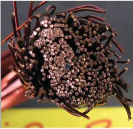
Dip & Bake Application Estimated 24% penetration of varnish
