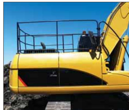
The engine bay of the excavator is fully enclosed by integrated guardrails, enabling safe pre-start checks and maintenance on site
