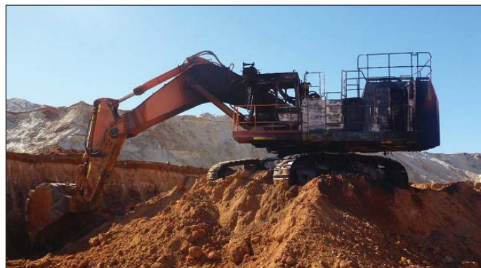
Photo 1 - Excavator after fire was extinguished
