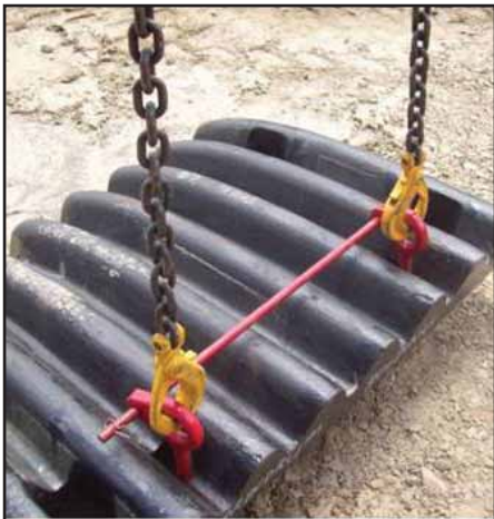
Lifting device using a pinned cross bar
