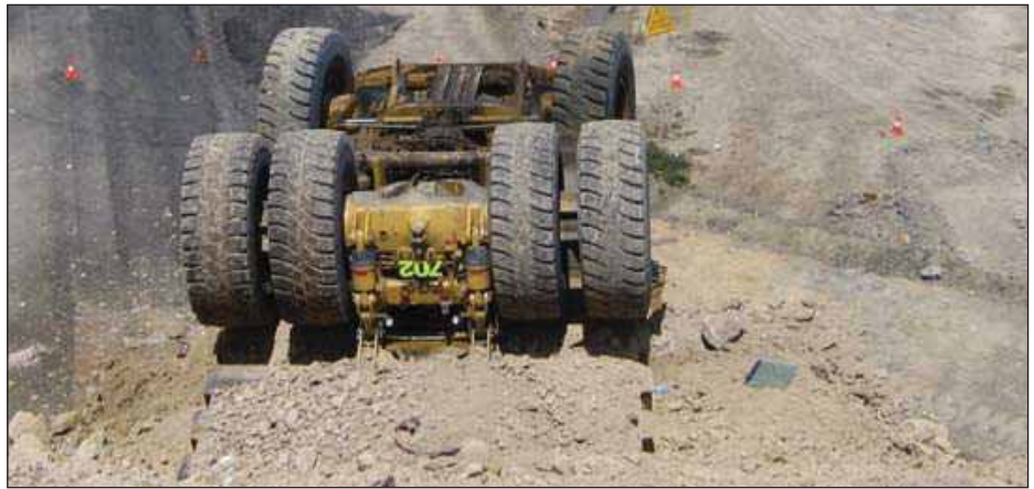
Haul Truck that toppled over the edge
