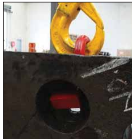
Lifting eye rotated into recess
