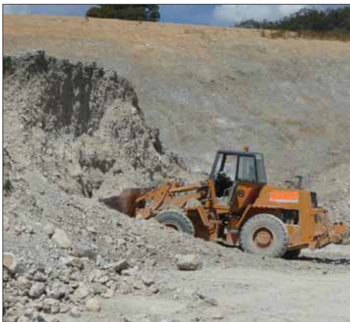
Shale and gravel from stockpile collapse into front end loader
