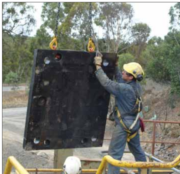
Mangasafe in action safely lifting a jaw liner
