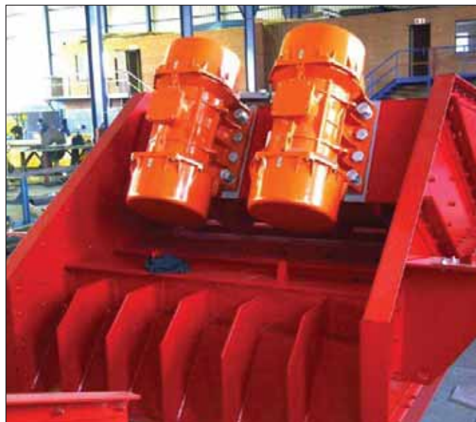
Large 8 pole vibrators connected to a Sizemack Screen
