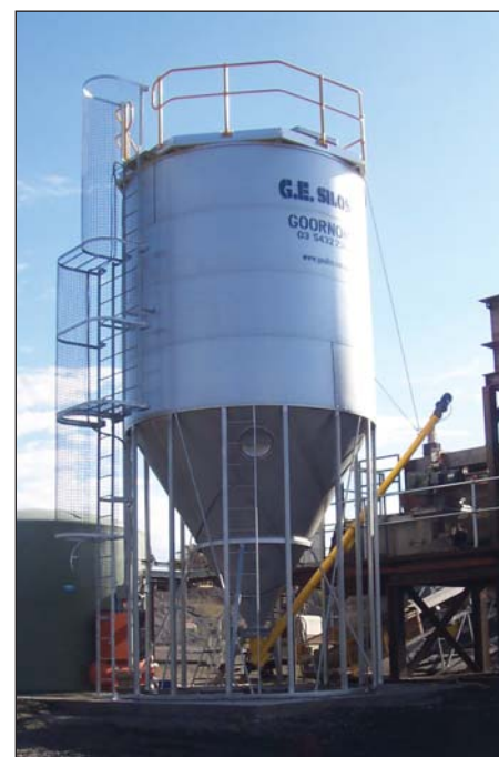
Claypro silo feeder
